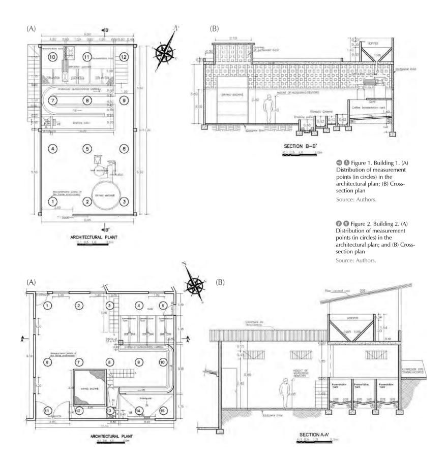
and the distribution of measurement points in the inside environment (in circles) of the three facilities for wet coffee processing. Figures 1(B), 2(B), and 3(B) show their cross-section plans.
