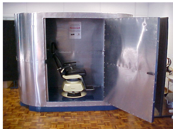
Figure 2. Faraday cage used in the experiments.
