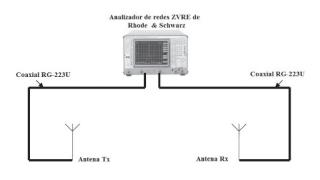
Figure 3. Measurement set up.
