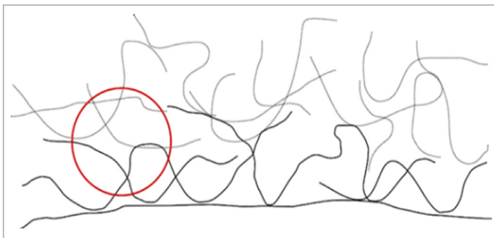
Figure 4. The hydrophobic modifications allow the polymer to build up because of the association of the hydrophobic groups, (SPE 165091) 3 .
