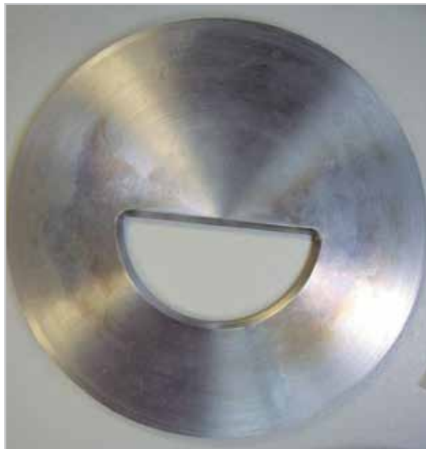
Figure 18. Back face view of a half moon orifice plate mimicking partial blockage of an orifice.
