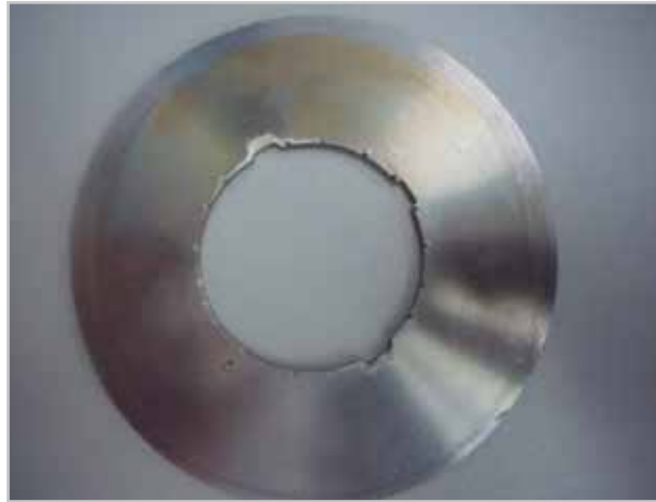
Figure 17. Damaged orifice plate.
