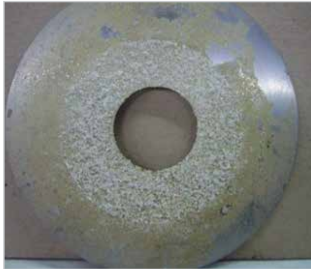
Figure 22. Contaminated orifice plate.
