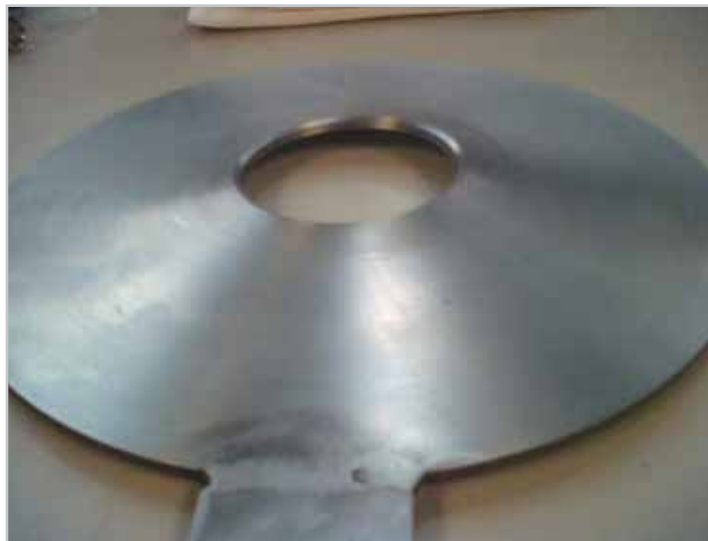
Figure 10. Buckled (or "Warped") orifice plate tested.
