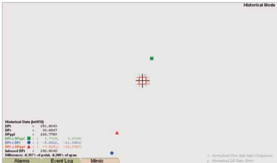
Figure 19. A partial blockage of the orifice.
