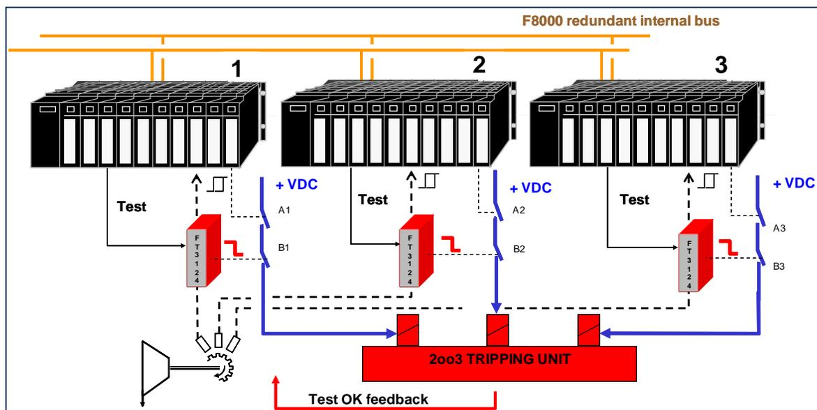
Fig. 1. 2oo3 Control System Architecture.
