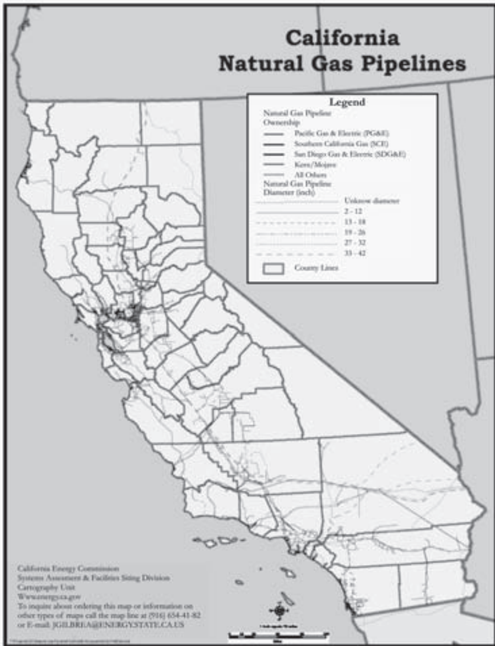
FIGURE 2. California existing natural gas pipelines and natural gas centers/hubs in relation to production basins and major flow corridors
