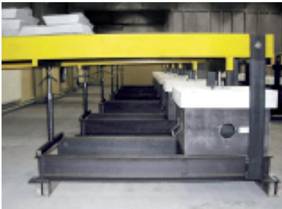
**Picture 7:** Creep test set up.
