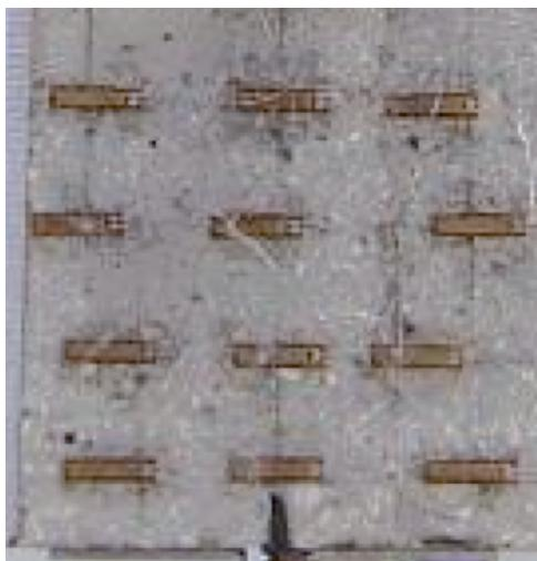
**Fig. 2.** Arrangement of stain gauges.
