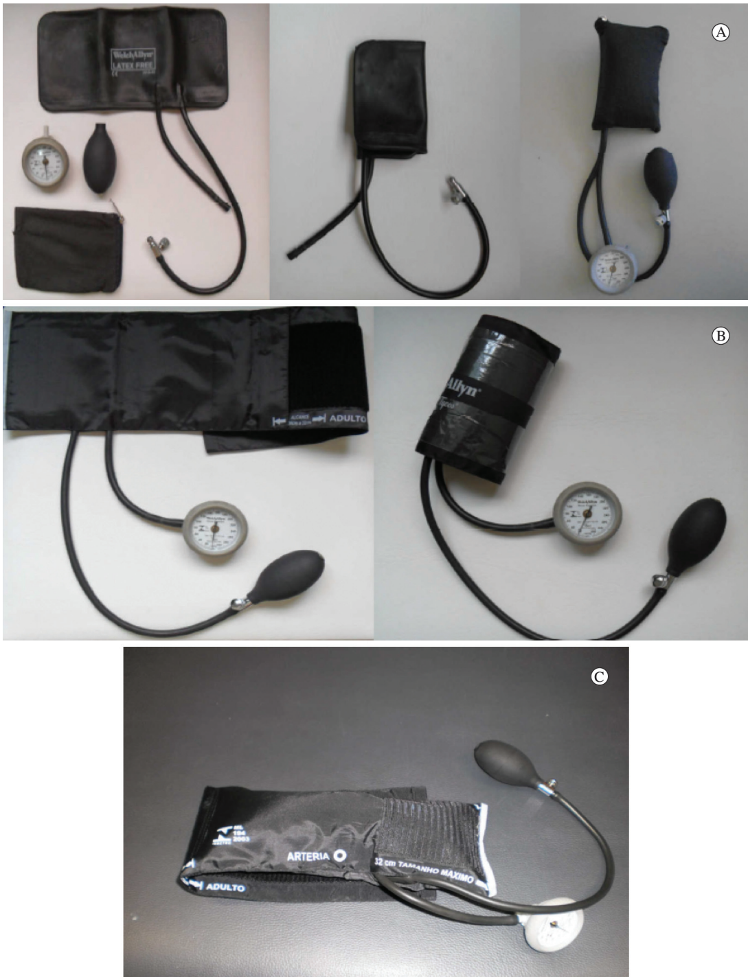
Figure 1. Sphygmomanometer adaptation methods for the assessment of muscular strength: (A) bag method; (B) cuff method; (C) without adaptation.
