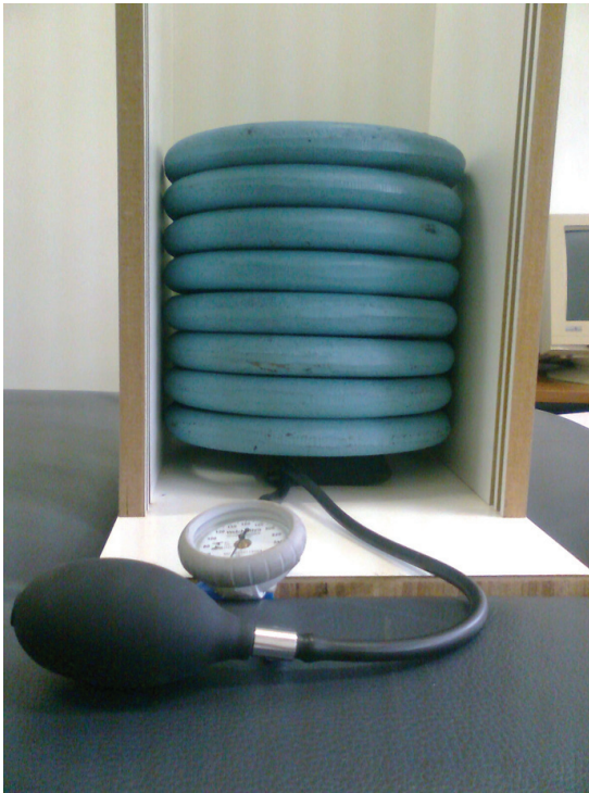
Figure 2. Apparatus for the calibration of the sphygmomanometer using 5 kg weights.
