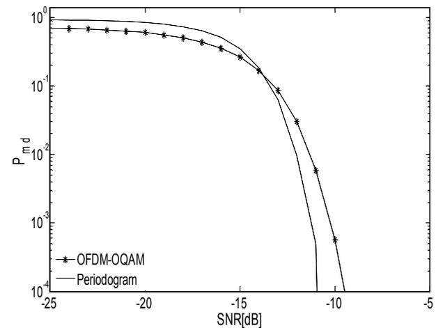
Fig. 3. Misdetection probability vs SNR for OFDM-OQAM and for the periodogram, with a fixed false alarm probability of 0.1 and a sensing time of 0.7 ms.
