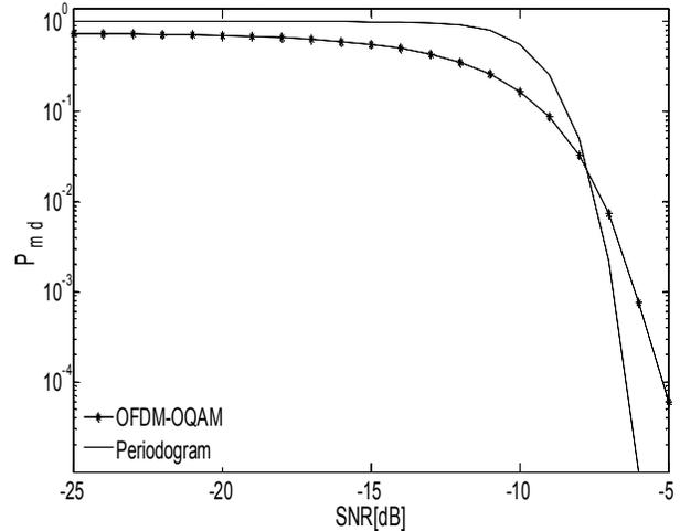
Fig. 2. Misdetection probability vs SNR for OFDM-OQAM and for the periodogram, with a fixed false alarm probability of 0.1 and a sensing time of 0.2 ms.
