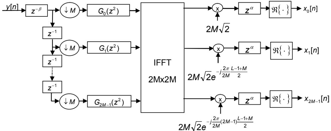
Fig.1. OFDM-OQAM demodulator
