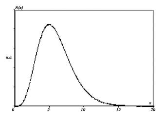
FIGURE 5. Plot of density of energy emitted by a black body.
