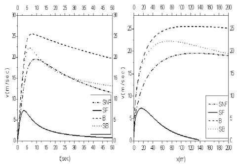
FIGURE 6. Plot in the v - t plane (left), and the v - x plane (right) when the objects run over an exponential trajectory with drag force.
