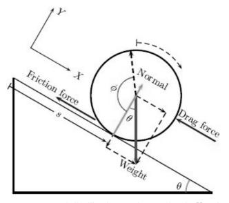
FIGURE 1. A snowball rolling downward on a wedge, the X-axis is parallel to the wedge surface and the Y-axis is perpendicular.
