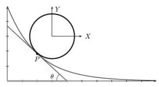
FIGURE 2. A snowball rolling downward on an exponential trajectory. To find the local value of the angle  $\theta$  we define the X, Y - axis as indicated in the figure. We see that for a sufficiently large value of x we get  $\theta \to 0$ .
