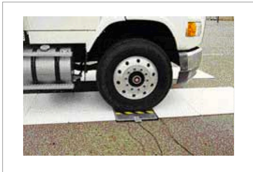
Figura 4. Sensor de capacitancia. Liu et al. (2006) Figure 4. Capacitance sensor. Liu et al. (2006)
