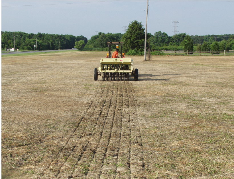
Figure 2. A truax drill seeded deposits meadow seed in a prepared seed bed providing good seed/soil contact.
