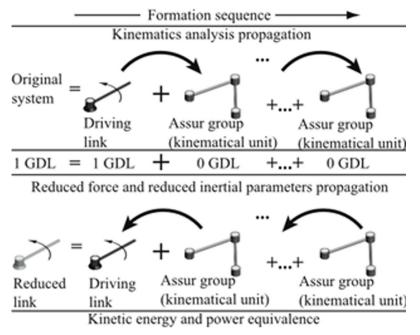
Figure 2. Modular propagation of the kinematic analysis and of the reduction of forces and inertial parameters in mechanisms.
