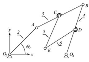
Figure 5. Case study, Watt's mechanism.
