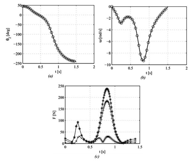
**Figure 6.** Forward dynamics of the case study's reduced link. a) Generalized coordinate  $(\theta_2)$ . b) Angular velocity  $(\omega)$ . c) Pair reactions (F). Convention for the figures a) and b): — modular dynamics;  $\bigcirc$  commercial MBS. Convention for the figure c):\* reaction in O2; + reaction in A; x reaction in E.
