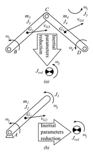
*Figure 4.* Inertial parameters reduction. *a*) In an Assur group with two links and three rotational pairs. *b*) In a driving link with fixed pivot A.
