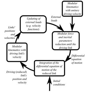
Figure 1. Modular dynamics of mechanisms.
