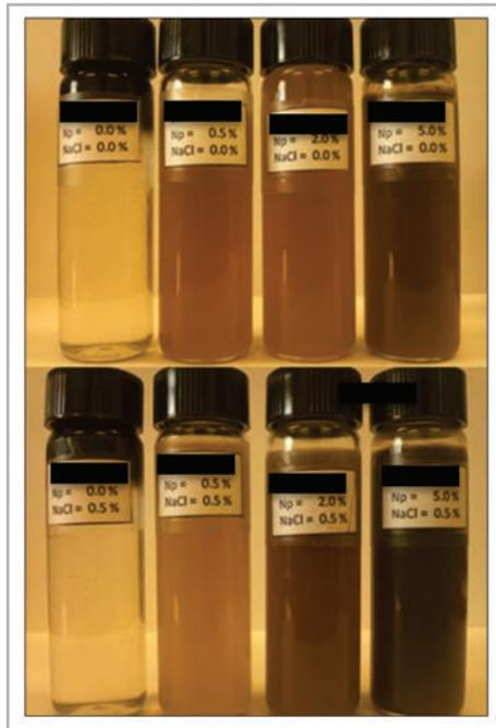
**Figure 1.1.** Samples of emulsions generated using deionized water and brine with heavy oil 1.
