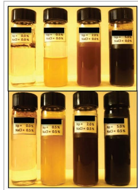
**Figure 1.2.** Sample of emulsions generated using deionized water and brine with heavy oil 2.
