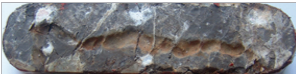
Figure 6. Core treated in laboratory showing an induced flow channel.
