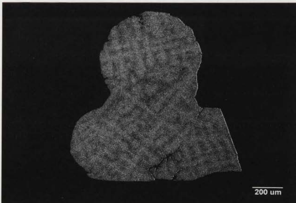
Photograph 6: SEM micrograph of a polished section through the broken tip of tunjo 7. Note the continuity of the cast structure between the base plate of the tunjo, running horizontally across the bottom of the photograph, and the round sectioned "wire" on top of it. [BSE image. Width of section 1.2 mm] [photo S. La Niece, British Museum].
