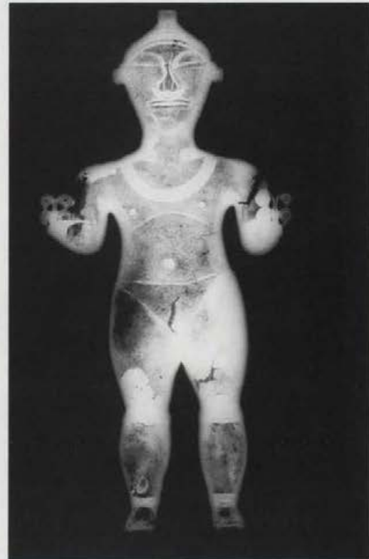
Photograph 9: Radiograph of the standing male lime-flask showing constructional details as well as casting faults and secondary casting runs (see text for interpretation) [S. La Niece, British Museum]
