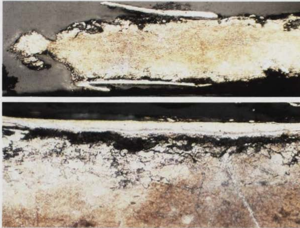
Figure 20a : Unetched cross-sectional view of part of the silver sheet of the spoon with a gold inlay over part of the surface. As polished; magnification x80.
