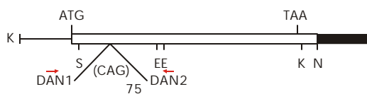
Figure 1. Configuration of the microinjection fragment used for transgenesis. The thin line depicts the 5' upstream regulatory region of the human SCA2 gene. The white box indicates the human full-length SCA2 cDNA with 75 CAG repeats. The black box indicates the poly(A) addition site from SV40. Primers for PCR DAN 1 and DAN 2 are indicated. Recognition sites for the restriction enzymes Kpn I, Sac I, Eco RI and Nhe I are also indicated as K, S, E, and N respectively.
